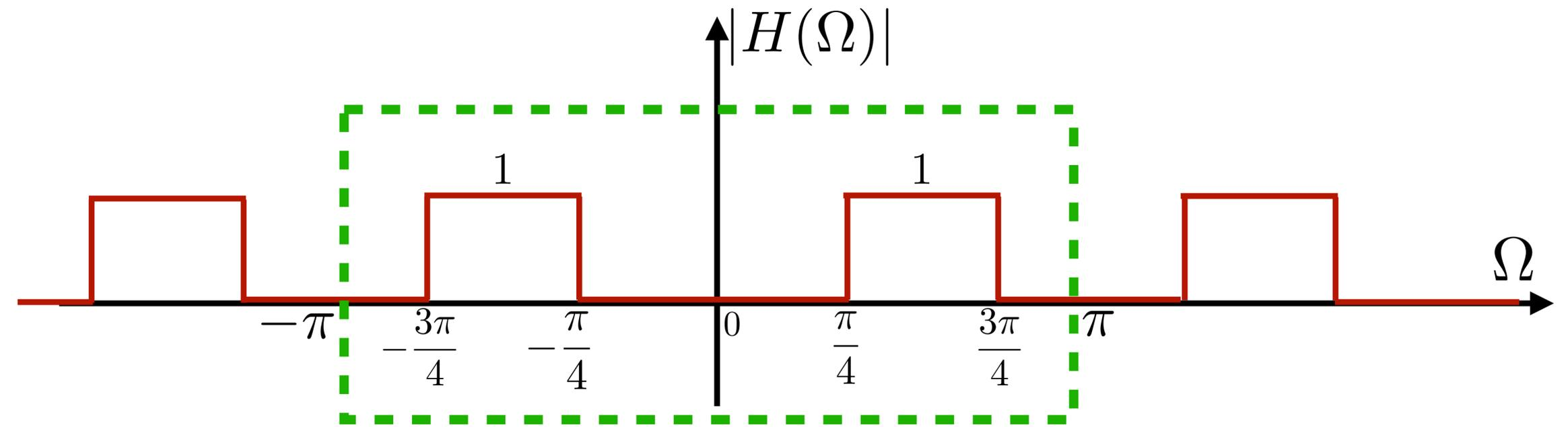
This is a band-pass filter. (proper explanation leave to the student but recall figure below)
