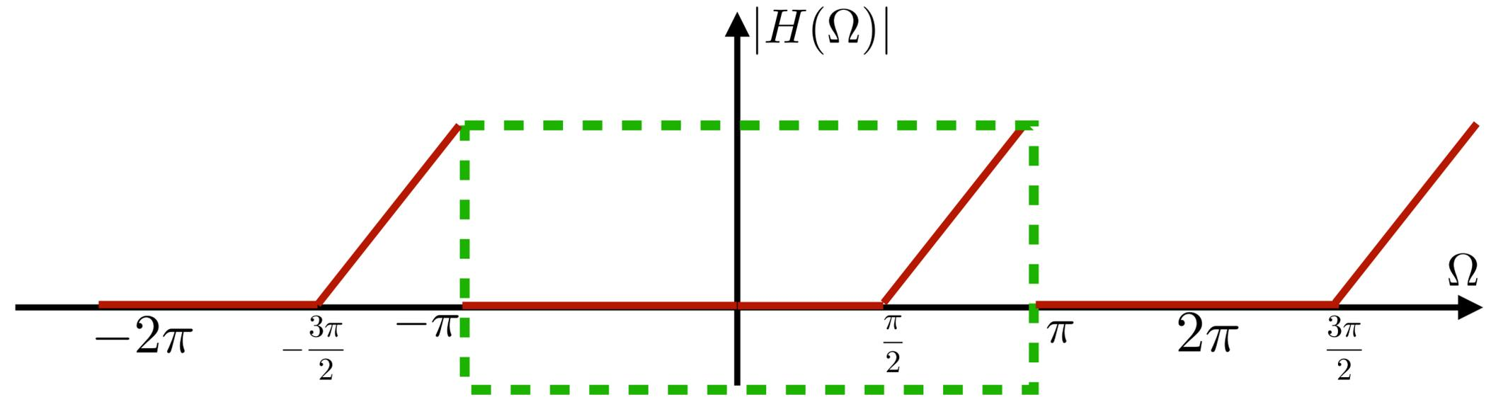
This is a high-pass filter. (proper explanation leave to the student but recall figure below)
