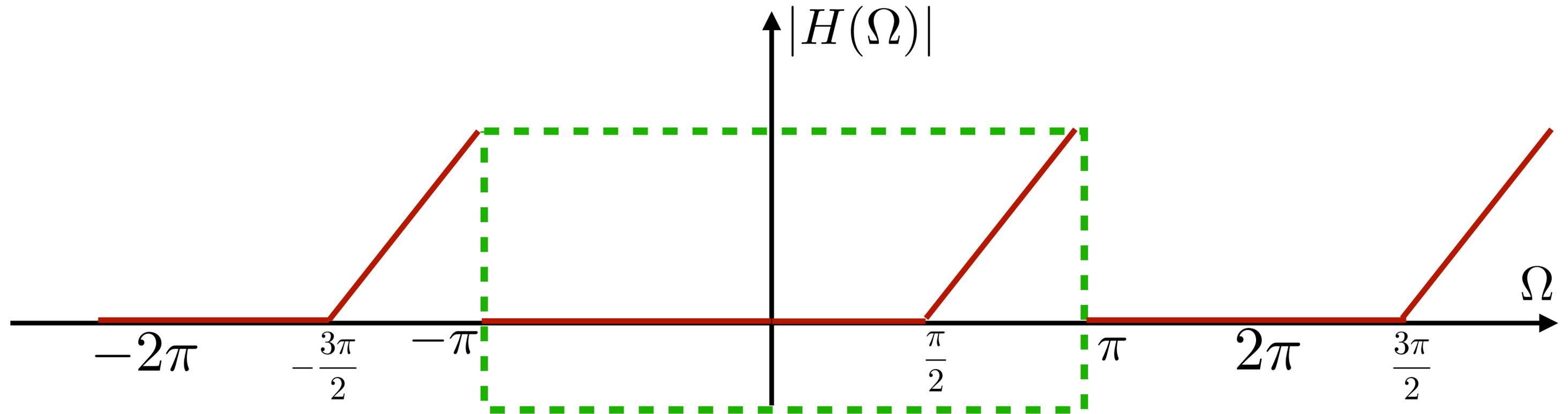
Say if it represents a low-pass filter, high-pass filter or a band-pass filter, and give a proper explanation.
