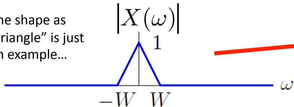
Signal with finite bandwidth:
