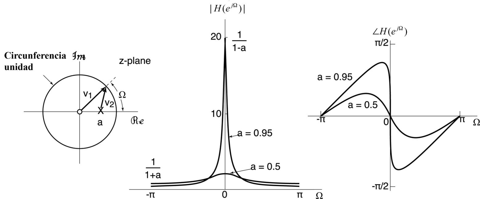
$$H(e^{j\Omega}) = \frac{v_1}{v_2}, \quad |H(e^{j\Omega})| = \frac{|v_1|}{|v_2|} = \frac{1}{|v_2|}, \quad \angle H(e^{j\Omega}) = \angle v_1 - \angle v_2 = \Omega - \angle v_2$$
